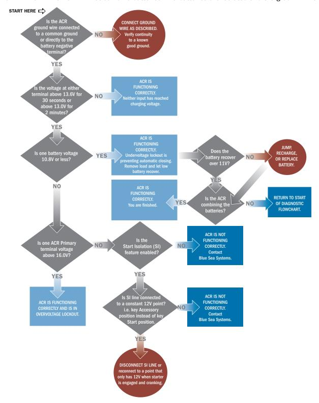
SYMPTOM The ACR will not isolate batteries. The batteries are combined and the green LED is ON.
