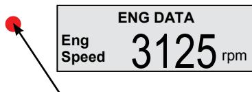
Illuminated red as long as any system faults remain active.
